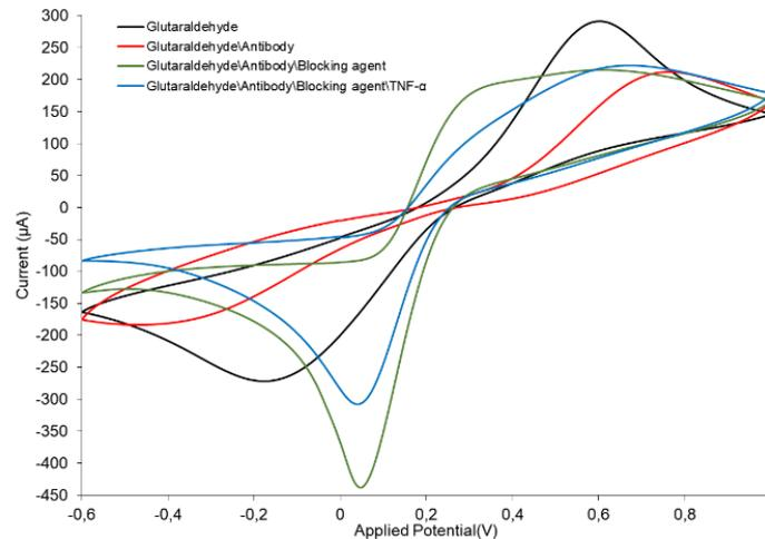
Figure 2. Characterization by cyclic voltammetry. (—) = glutaraldehyde, (—) = glutaraldehyde/monoclonal antibody, (—) = glutaraldehyde/monoclonal antibody/blocking agent, (—) = glutaraldehyde/monoclonal antibody/blocking agent/human TNF- $\alpha$ .
