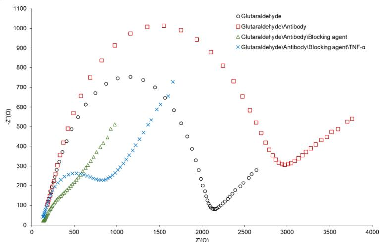
Figure 3. Characterization of the layers by EIS. (×) = glutaraldehyde, (+) = glutaraldehyde/monoclonal antibody, (◇) = glutaraldehyde/monoclonal antibody/blocking agent (○) = glutaraldehyde/monoclonal antibody/ blocking agent /human TNF- $\alpha$ .
