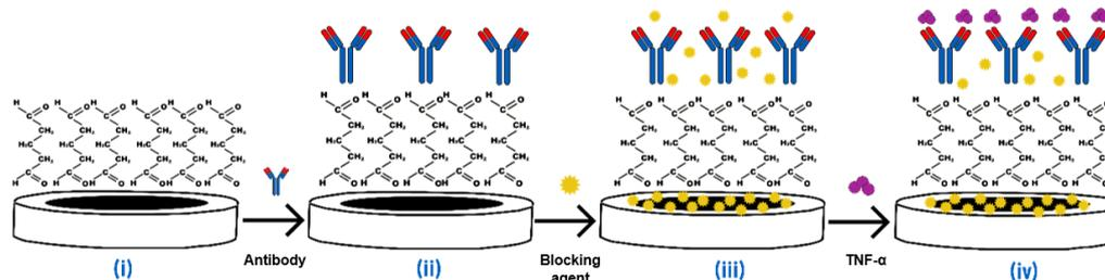
Figure 1. Steps in the production of the immunosensor for quantification of TNF- $\alpha$  using a carbon-paste electrode: (i) carbon-paste electrode modified with glutaraldehyde; (ii) immobilization of the monoclonal antibody; (iii) addition of the blocking agent to prevent non-specific binding; (iv) addition of TNF- $\alpha$ , the cytokine of interest.
