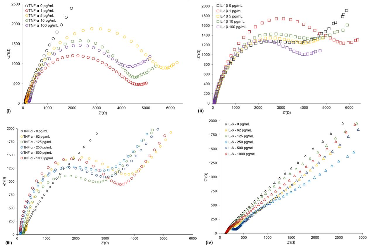
Figure 4. Assays in standard solution: (i) assays with TNF- $\alpha$  and (ii) assays with IL-1 $\beta$ , both in  $3 \text{ mol}\cdot\text{L}^{-1}$  solution of KCl with concentrations varying from 1 to  $100 \text{ pg}\cdot\text{mL}^{-1}$ ; (iii) assays with TNF- $\alpha$  and (iv) assays with IL-6, both in PBS pH 7.4 and with concentrations varying from 62 to  $1000 \text{ pg}\cdot\text{mL}^{-1}$ .
