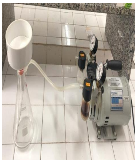
Figure 3 - Previous Washing System for the formed compounds
